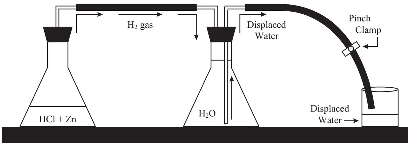
2. Measure out 100 ml of 6.0 molar HCl solution and place in leftmost flask.
